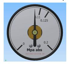
SF6 monitoring in MV Equipment was based on simple manometers based on bourdon tube element
