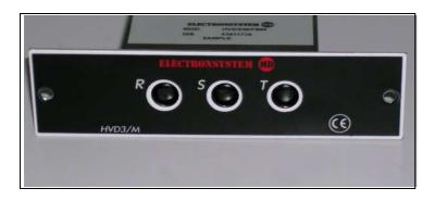
This VDS is based on the sharing of voltage between capacitor C1 (high voltage) and capacitor C2 (low voltage); the signal at C2 terminals is transformed in an optical signal, which separately points out voltage and phase of the line involved.
